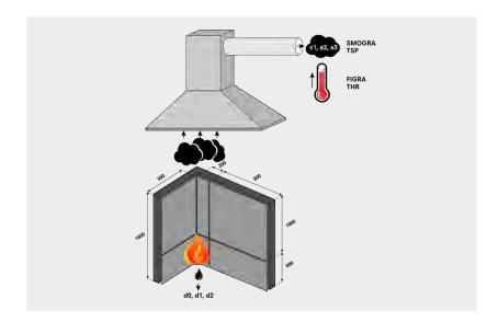
The classification parameters of the SBI test are fire growth rate index (FIGRA), lateral flame spread (LFS), and total heat release (THR600s). Additional classification parameters are defined for smoke production as smoke growth rate index (SMOGRA) and total smoke production (TSP600s), and for flaming droplets and particles according to their occurrence during the first 600 seconds of the test.
