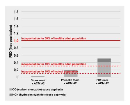
Contribution of CO, HCN,  $CO_2$  and lack of  $O_2$  to lethality (ISO 13344) at 30 minutes for gases entering a  $50 \, \mathrm{m}^3$  room from cladding through 100mm vent:
